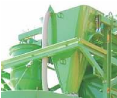
Separate cement and water weigher
