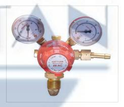
**C. Gas Regulators (Argon);** These are Double Stage Double Gauge Argon Gas Pressure Regulators having Inlet Pressure 0-300 bar and Outlet Pressure 0-10 bar. The Inlet Connection is 3/4"BSP(R/H) F & Outlet Connection 3/8"BSP(R/H)M. These have the Flow rates 60mÃ, ³/h(1000lit/min). They are used for Mig & Tig Welding purpose and conforms to the Standards IS 6901:2009.
